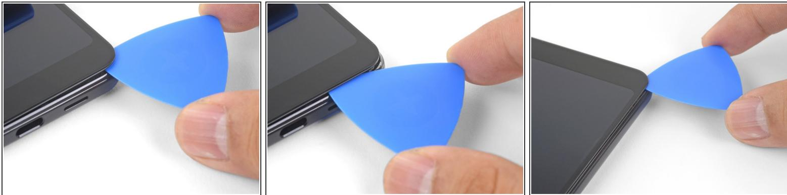
ⓘ As you slice around the bottom edge of the phone, do not insert the pick more than 1/4" (6 mm).
