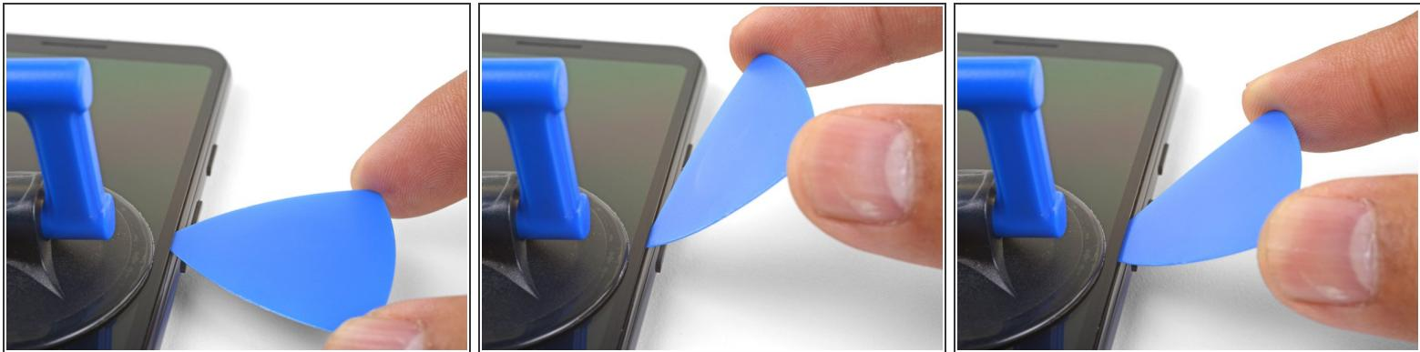
ⓘ This step shows how to insert the pick without damaging the LCD panel. Do this before you slice either long edges of the phone.
