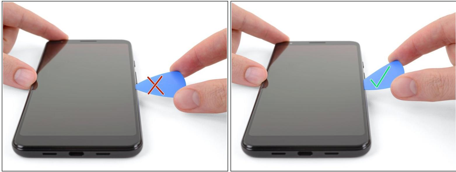
*(i)* In the next step you will insert an opening pick between the screen and the plastic body of the phone.
