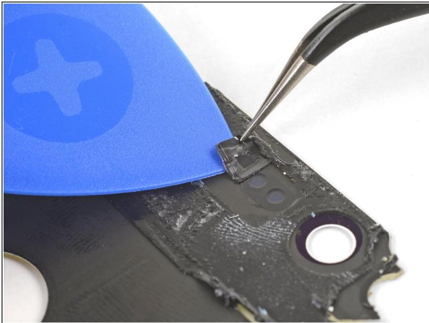
**i** If your replacement rear glass does not come with a microphone mesh, you will have to transfer the original over.
