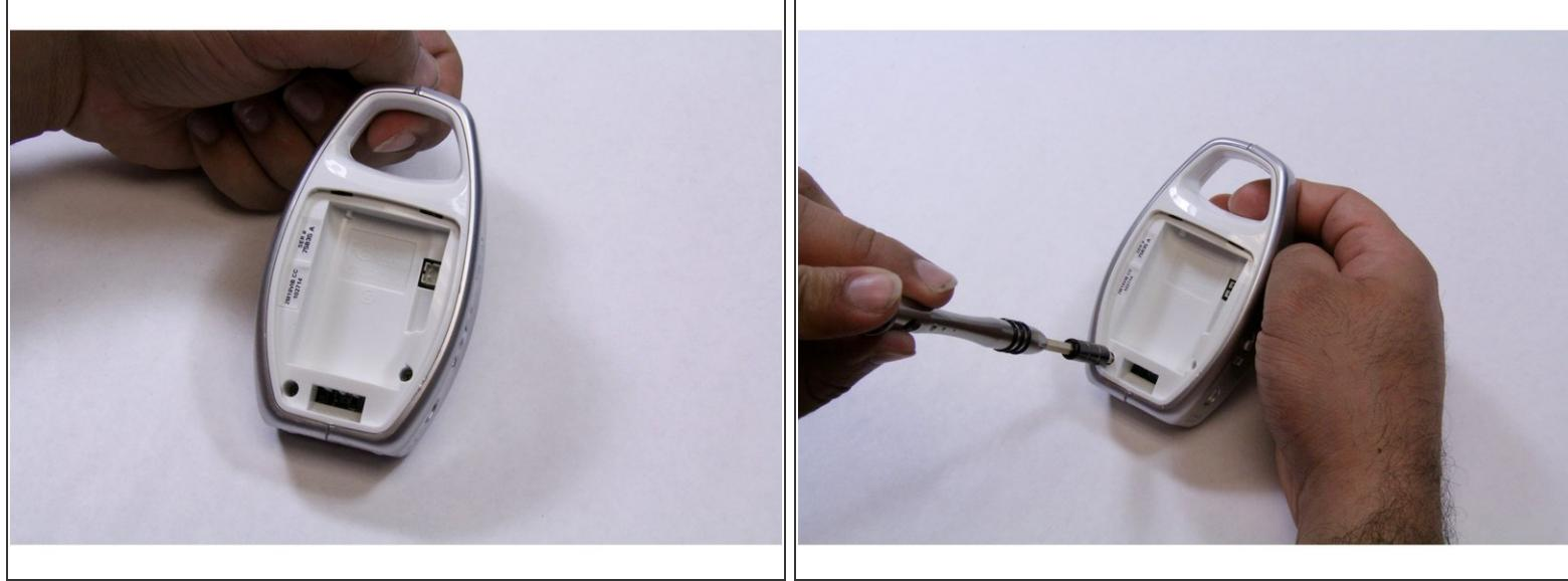
*(i)* There are two screws on the rare case of the device. For the one shown in blue marker requires either an extended screwdriver or putting on a little pressure on a regular screwdriver.
