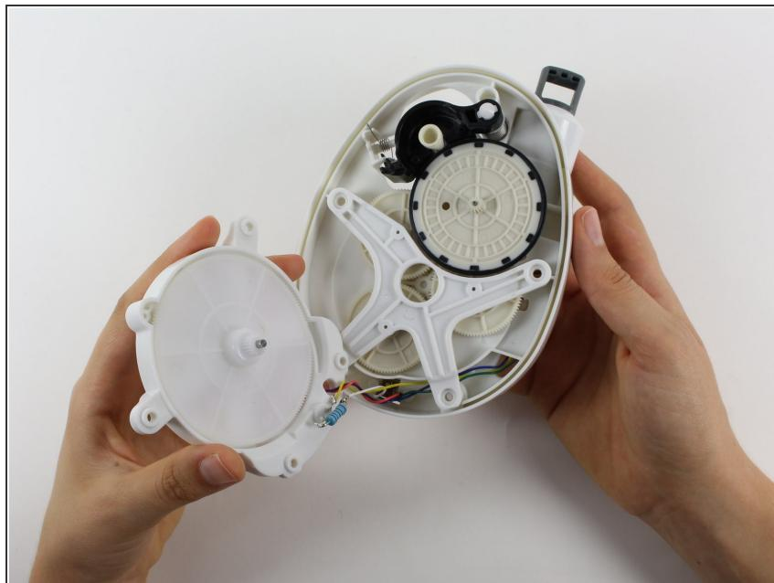
⚠ Watch out for the wires! Keep them attached for this entire guide, or the GravityLight will not work!
