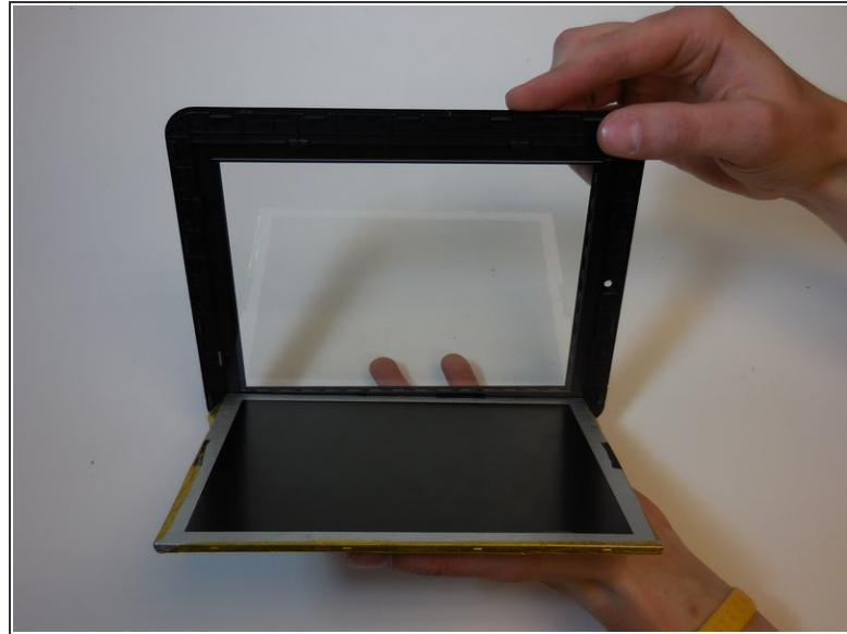
**i** The matrix is the component that is attached to the LCD (component with the silver backing). It is the component that interprets the location of the users touch.
