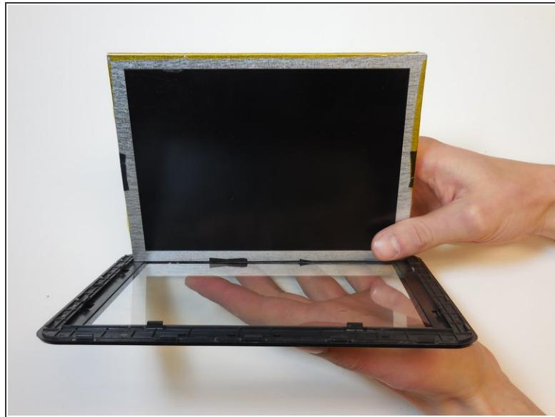
**⚠** The screen assembly is a delicate component and some prying is involved. Avoid deforming screen to avoid further damage.
