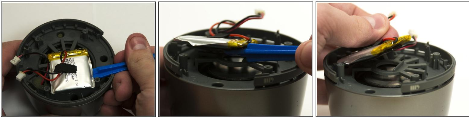
**⚠** Batteries can be very dangerous if punctured. Use extra caution when using tools around the battery.
