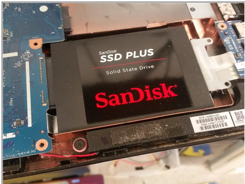
*(i)* Normally, there will be two screws holding the hard drive (or, in this case, solid state drive) in, but in this case, the screws are missing, and the SSD slid out from the connector.
