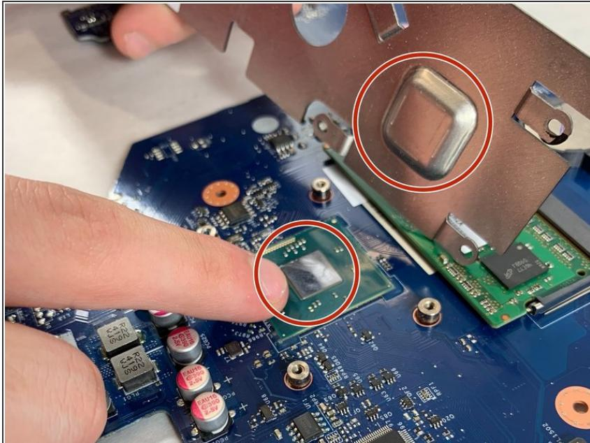
Before reconnecting the cooling fan assembly, make sure to [properly apply thermal paste](#) and touch the two connectors together when reassembling your laptop.
