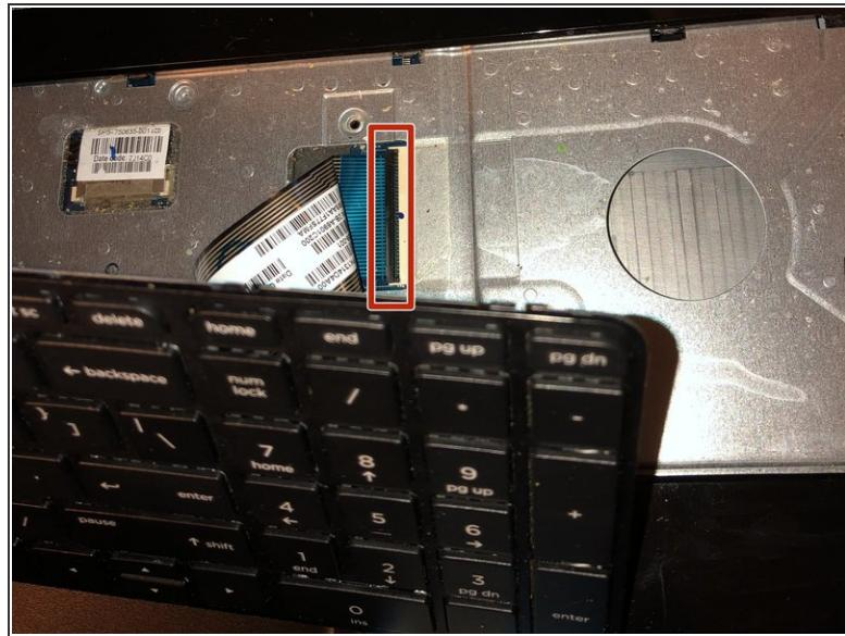
**⚠** Once the keyboard is loose, do not immediately pull away from computer. It is attached by the ribbon connector.
