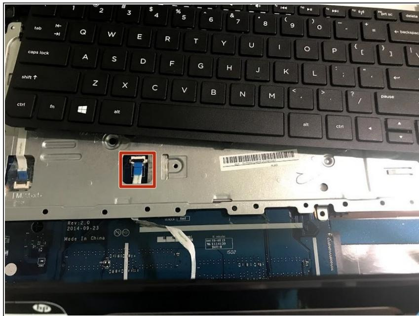
**⚠** The connection for the track pad is still connected.
