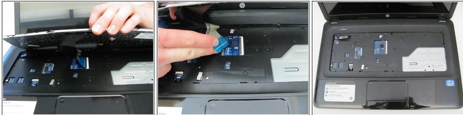
**⚠** Do not try to remove the keyboard immediately. It is still connected to the motherboard by a ribbon cable that can be easily damaged.
