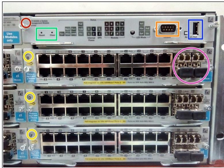
ⓘ The equipment comes with two modules to install a supervisor card and 6 expansion slots for compatible modules.
