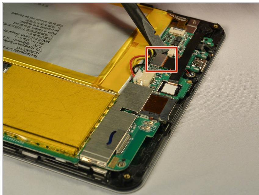
**i** The cameras are connected together via a small ribbon cable with one electrical connection in between them.
