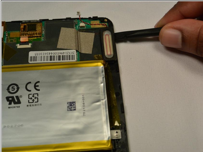
**i** A thin strip of double sided tape secure the speaker to the device and is located beneath the speaker.
