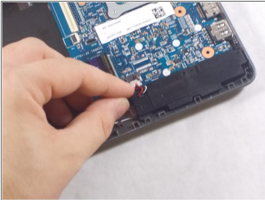
**⚠** Make sure to hold the white part of the plug and not the wire. If unplugged by holding the wires, it can rip out wires.
