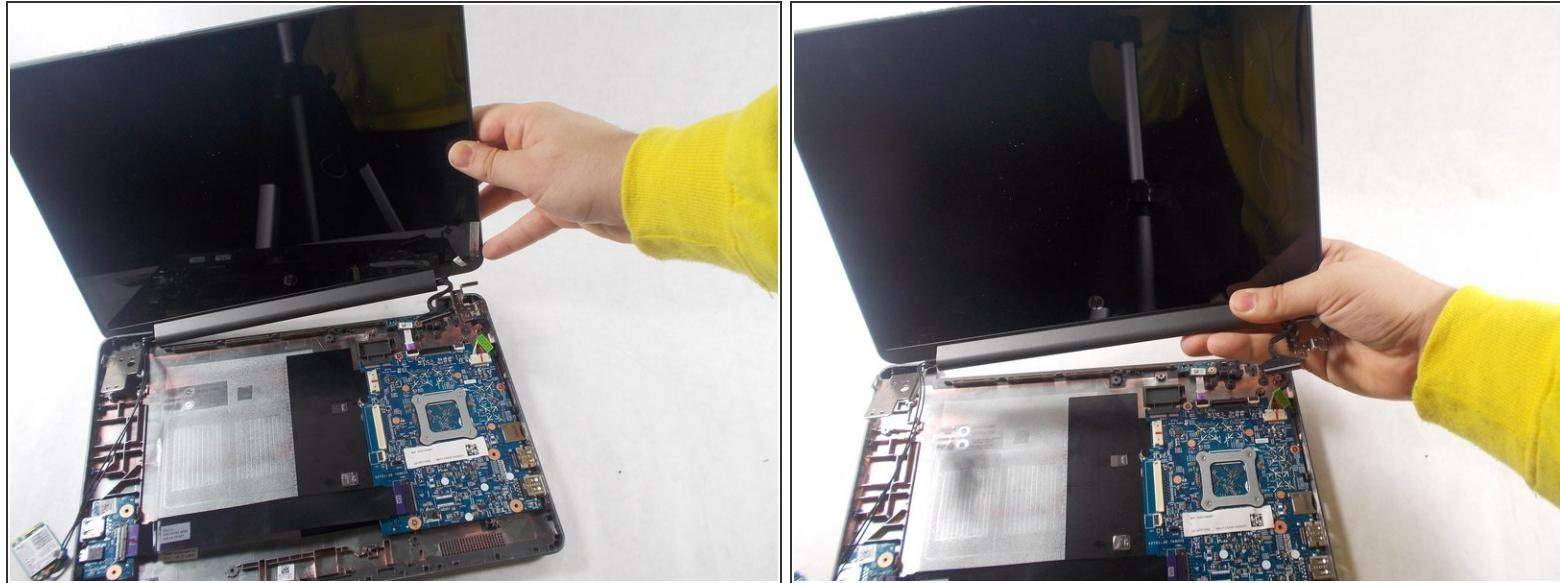
⚠ Be careful when removing the screen so it doesn't get caught on any wires.
