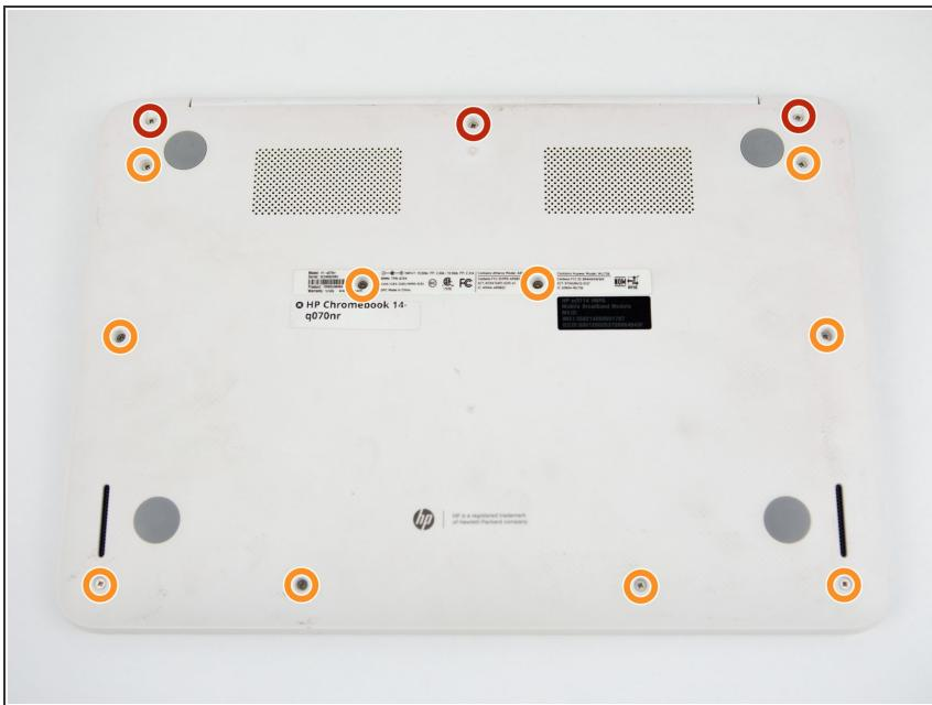
At this point, the white caps that hide the top-most screws marked with red circles have been removed.
