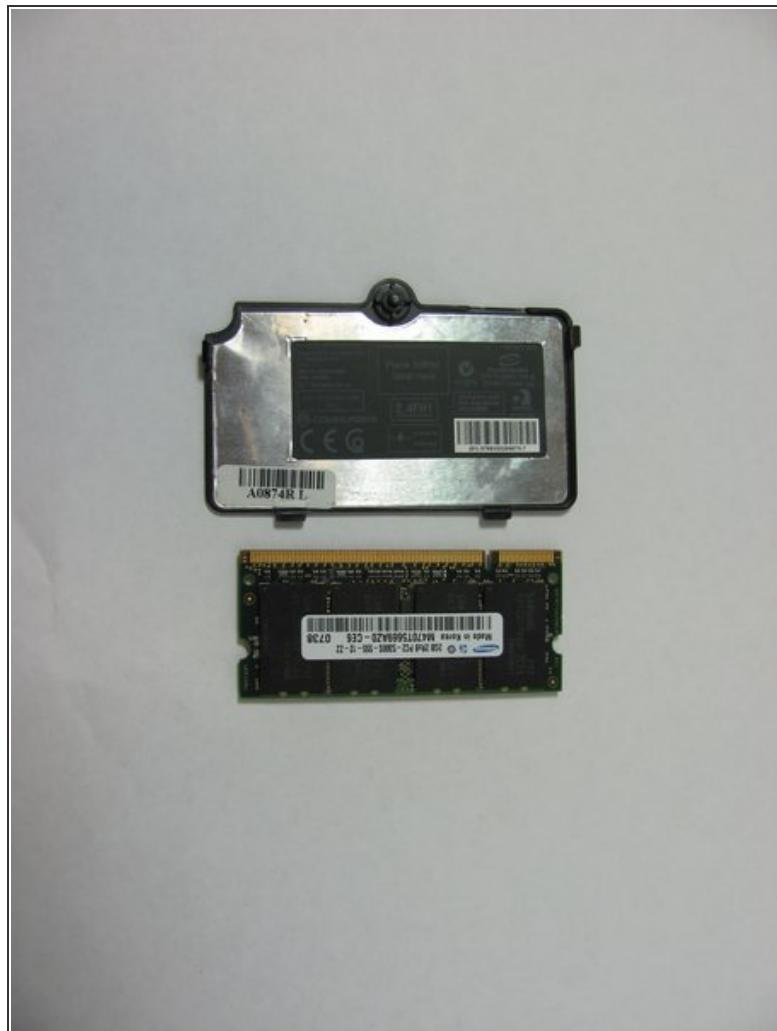
**⚠** The RAM chip is susceptible to static electricity. Before grabbing the RAM chip, make sure you have discharged the electricity from your hands by touching a metal surface other than your computer.
