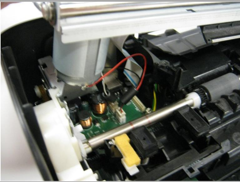
! Lift the rail carefully as a strip and motor will be connected to the bottom part of the printer.
