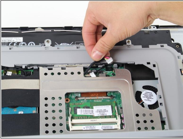
**⚠** Before working on any of the internal components of the computer, make sure the battery is disconnected so there's no power running through the device.
