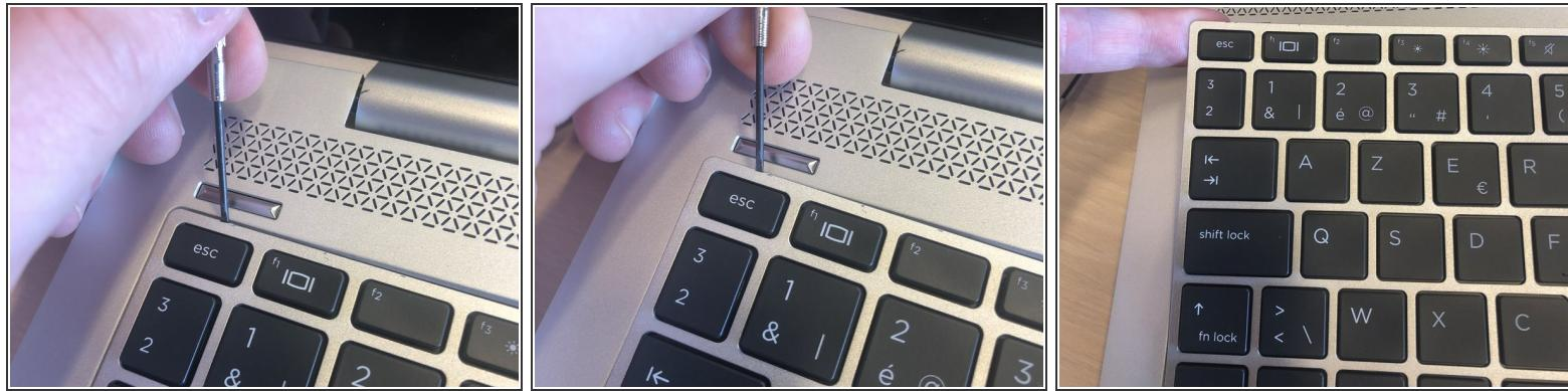
**⚠** I recommend to use the **iFixit Opening Picks** for this step! Otherwise you could scratch/damage the keyboard or frame by metal on metal!
