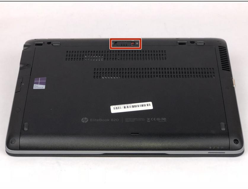
**!** Ensure the laptop is completely powered off and power adapter is unplugged before removing the battery.
