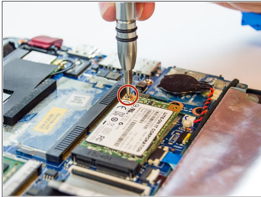
ⓘ After removing the cover the mSATA SSD should be visible near the center of the device.
