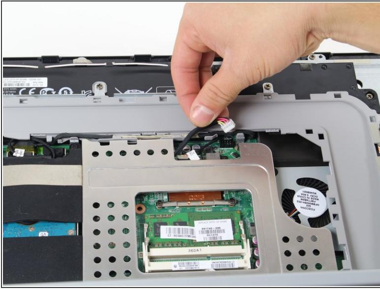
**⚠** Before working on any of the internal components of the computer, make sure the battery is disconnected so there's no power running through the device.
