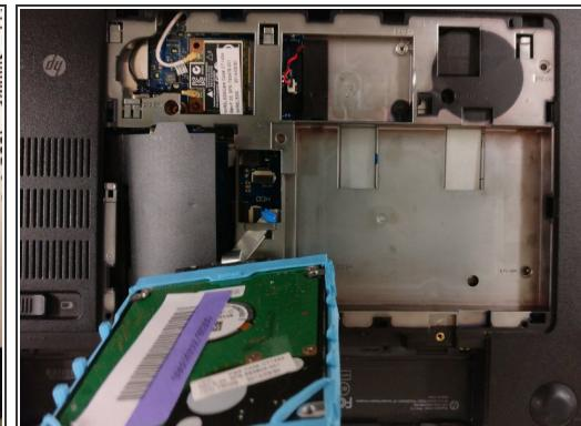
ⓘ The hard drive is connected to the motherboard via this blue-tabbed cable, highlighted in red.
