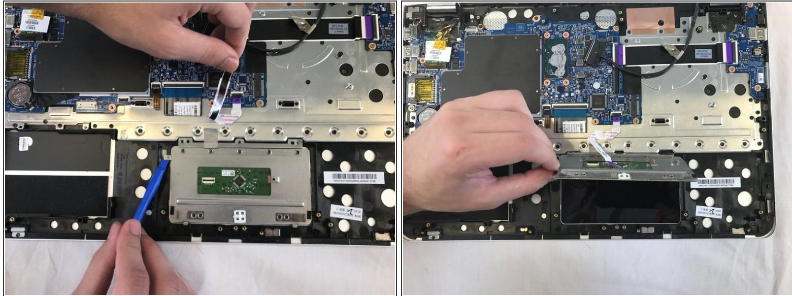
*(i)* Keep the ribbon cable from interfering with touchpad removal.
