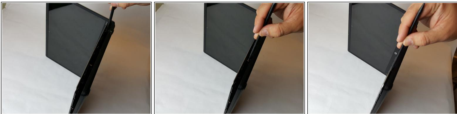
**ⓘ** This step requires unlocking the very fragile plastic clips along the frame; take care not to damage them.
