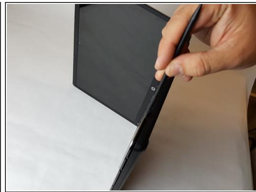
**ⓘ** This step requires unlocking the very fragile plastic clips along the frame; take care not to damage them.
