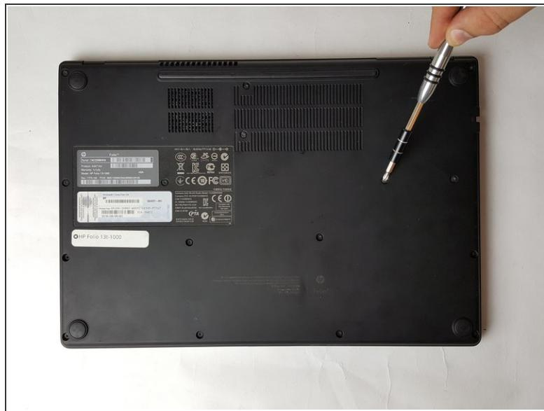
**⚠** Use an antistatic wrist wrap, or periodically touch unpainted metal to minimize the risk of damaging the laptop by electrostatic shock.
