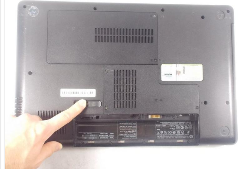
⚠ Make sure to turn off the laptop before removing the battery.
