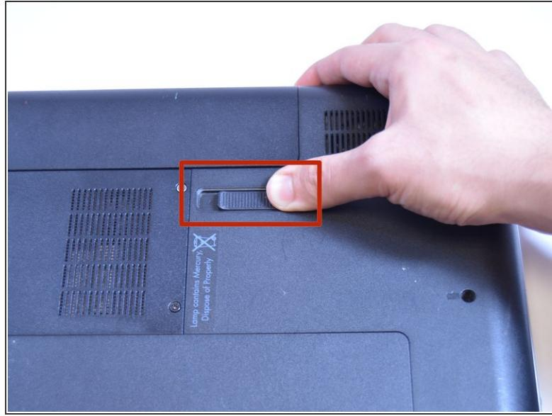
! Removing the battery while the laptop is still on may corrupt your files.
