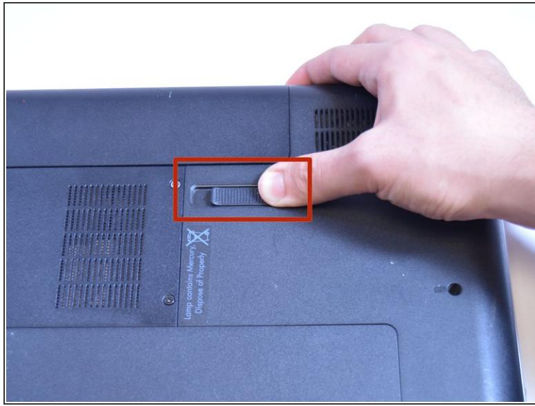
! Removing the battery while the laptop is still on may corrupt your files.
