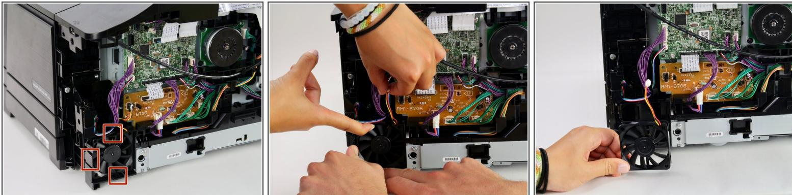
ⓘ There are three tabs that hold the fan in place, as shown in the first picture. These steps may require an extra pair of hands in order to depress all the tabs.
