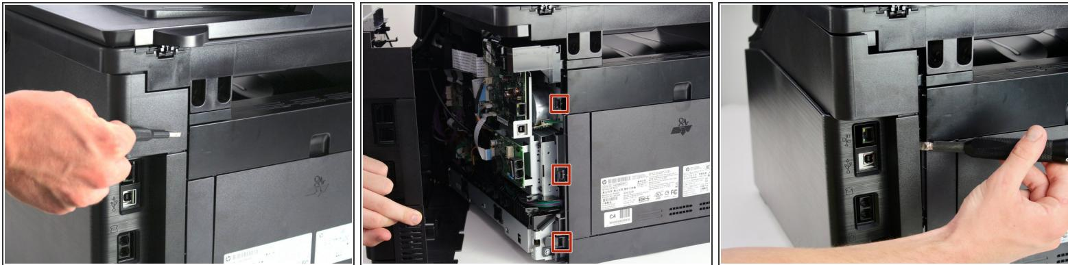
ⓘ There are three tabs along the back right corner of the printer underneath the panel shown (location is displayed in second picture).
