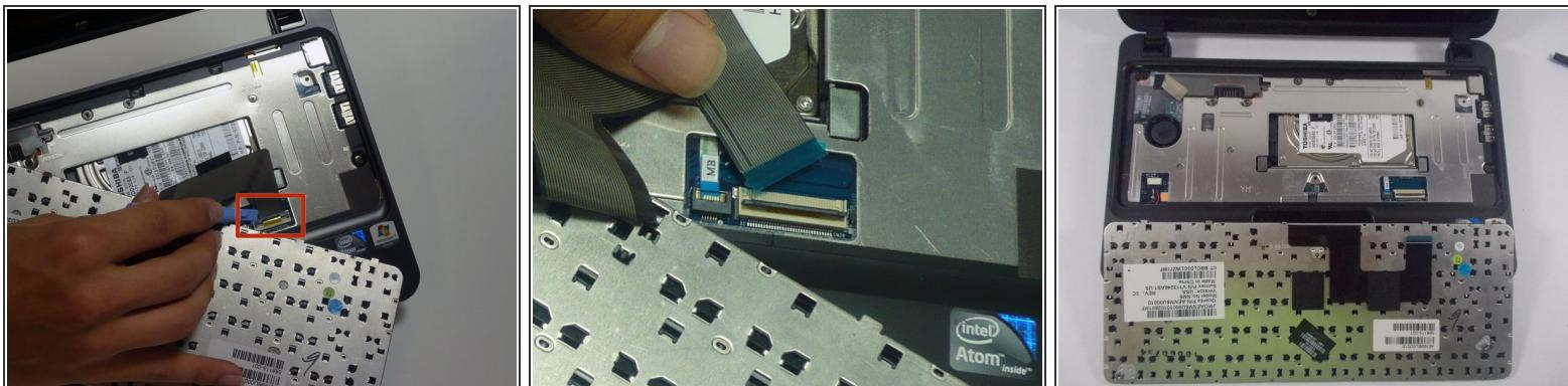
⚠ Be very gentle with the ZIF connector! It is designed to be locked into the motherboard, so make sure you lift the retaining latch before attempting to disconnect it.
