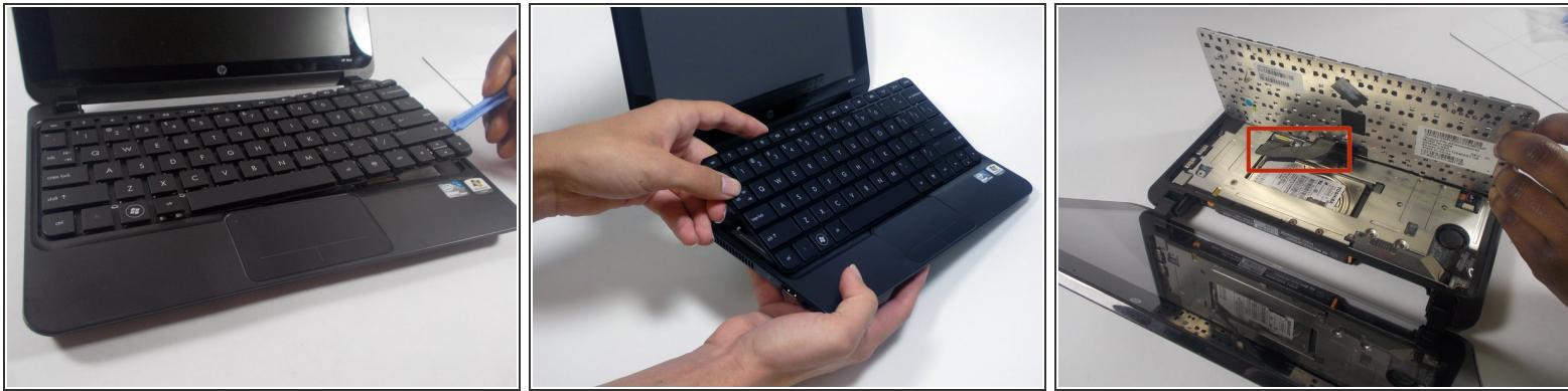
ⓘ After removing the plastic casing surrounding the keys, carefully lift the full keyboard from the netbook using a plastic opening tool.
