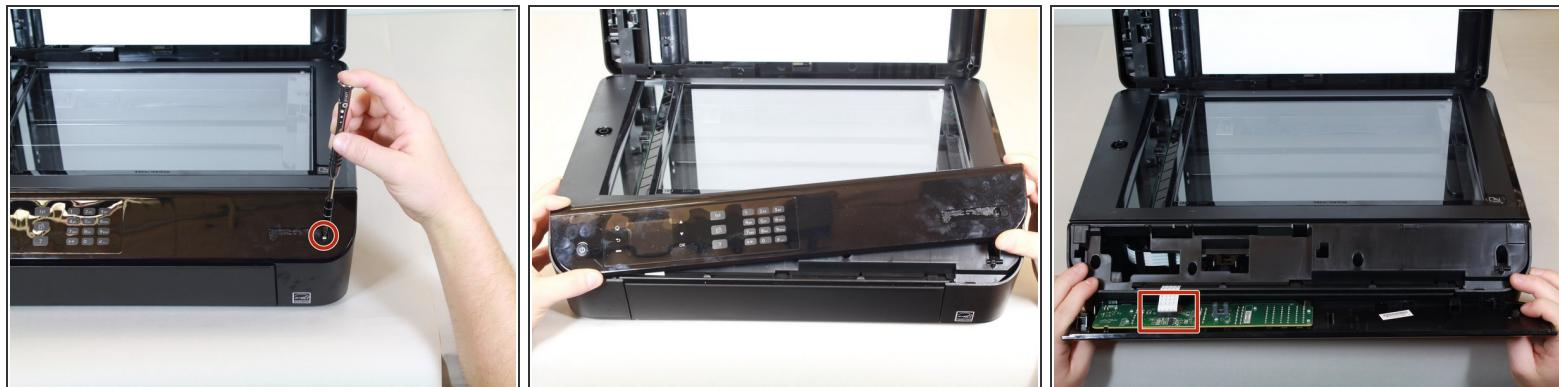
● Remove the single 12mm-T10 screw securing the front panel to the printer body.
