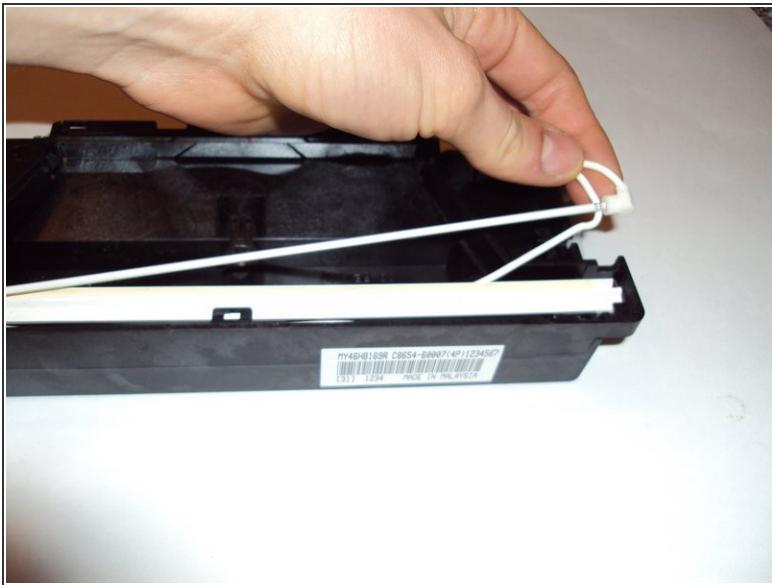
**⚠ Carefully** twist white scanner lamp support out of its carriage and replace it with a new one.
