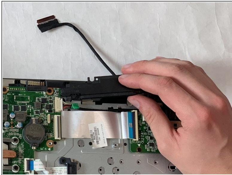
**⚠** Disconnect wiring harnesses by gently applying pressure to the plastic clip. Do not pull on the wires.
