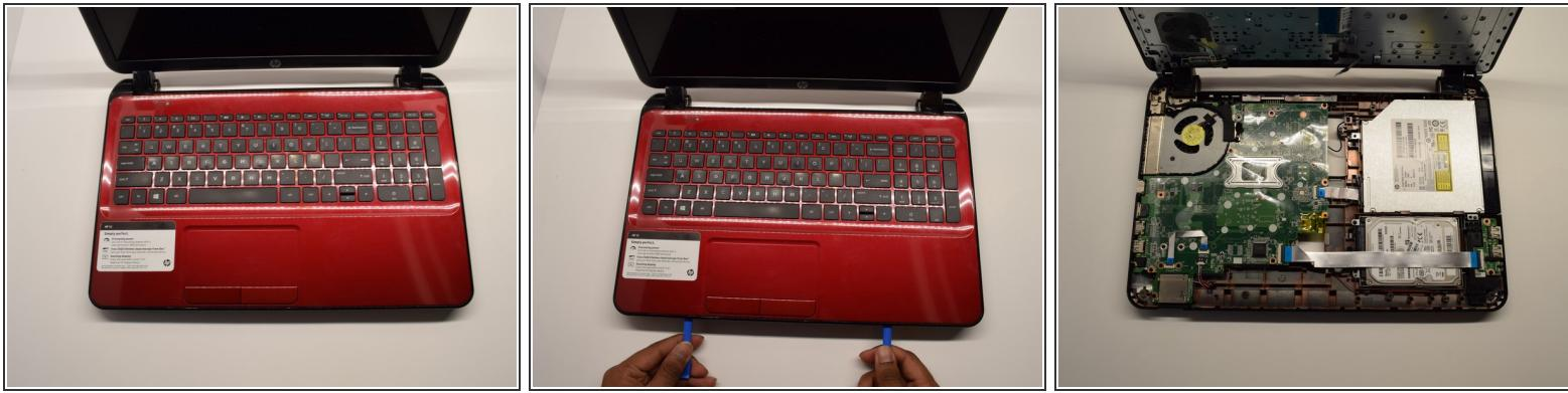
ⓘ Flip the computer over so the screen and keyboard are showing.
