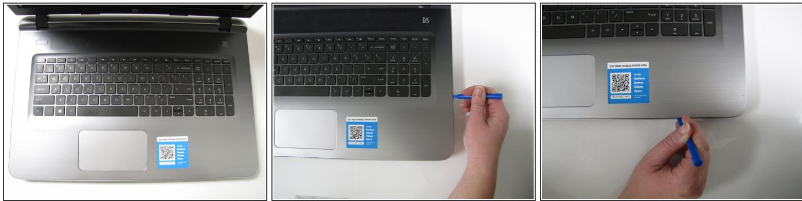
**⚠** Make sure that all screws and the CD-ROM Drive are removed before trying to complete this step to prevent damaging your laptop. During this step, you will likely hear loud crackling noises. This is normal.
