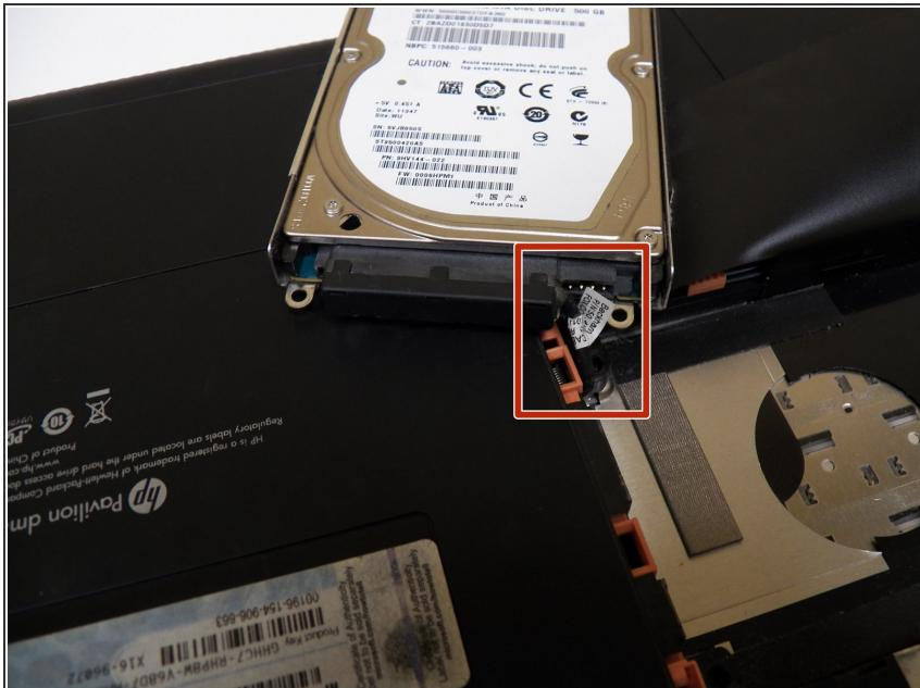
**!** Pay attention to the SATA cable connecting the hard drive to the motherboard. It can be damaged if handled roughly.
