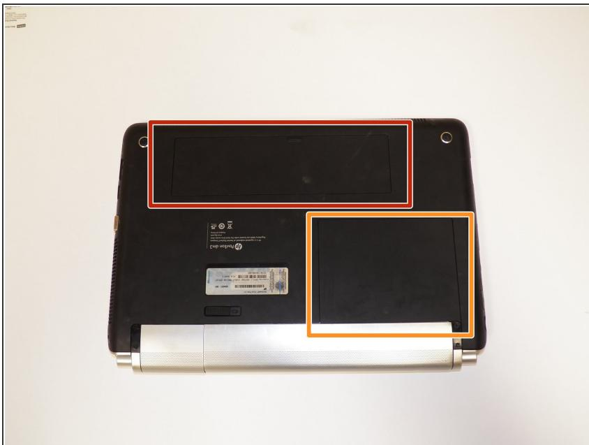
ⓘ Remove the 2 plastic panels covering the internals of the laptop.
