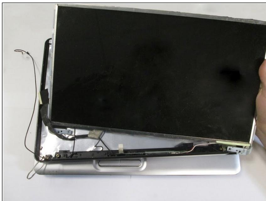
⚠ Be careful when moving the screen, you may damage the monitor and webcam cable.
