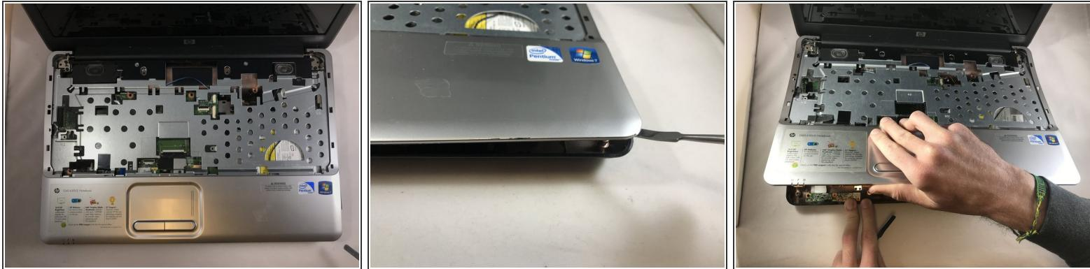
ⓘ In order to be able to unplug the cables that connect the screen to the motherboard, we will need to remove the metal support.
