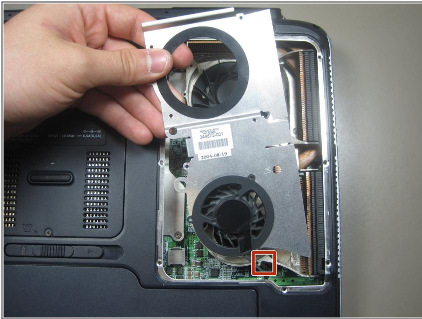
**⚠** Lift the plate and lower fan off the heat sink being careful not to damage the lower fan cable, which is attached to the motherboard.
