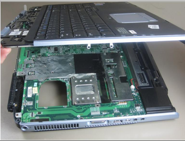
⚠ Do not remove the keyboard yet! There are still wires connecting the two components.
