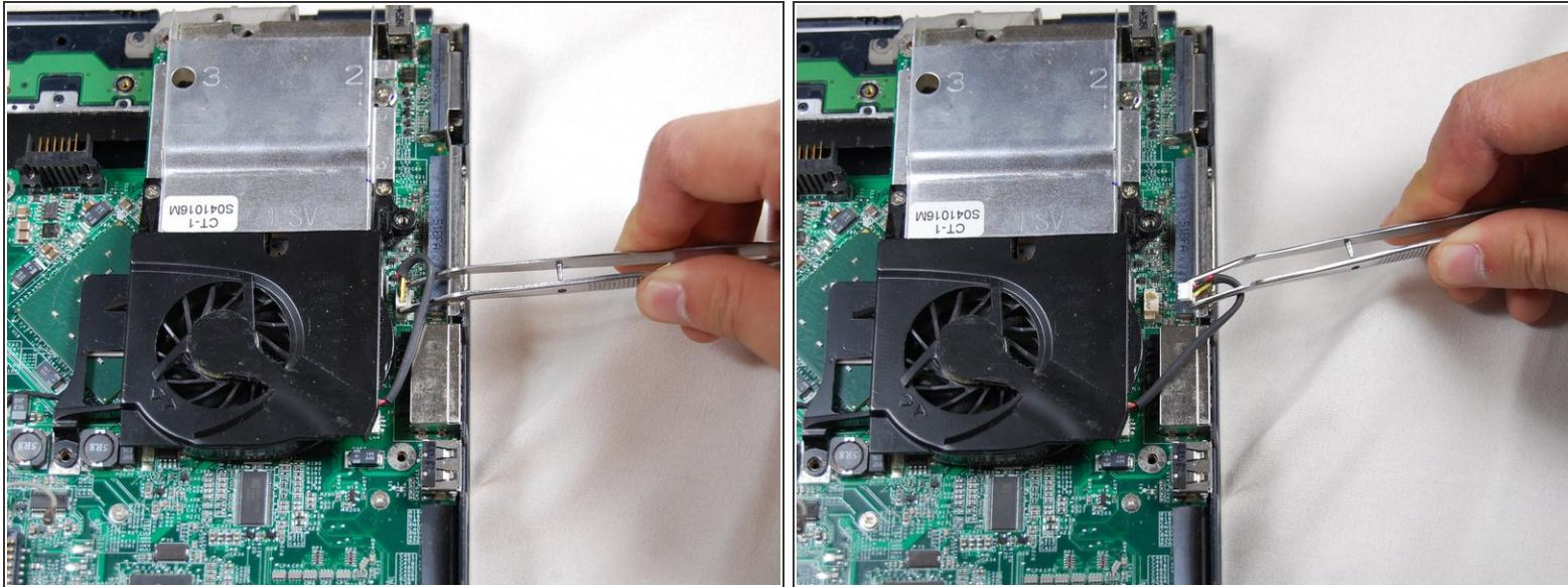
**⚠** After removing the screw, use your tweezers to remove the wire connecting the fan to the board. Do not pull the fan out immediately or it may damage the fan and/or the computer.
