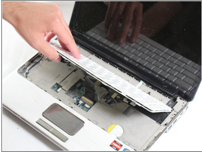
⚠ Underneath the keyboard there is a flat cable that connects the keyboard to the computer. Do not remove the whole keyboard just yet because there is a cable that has to be detached first. If the keyboard is pulled too hard, the cable may rip.
