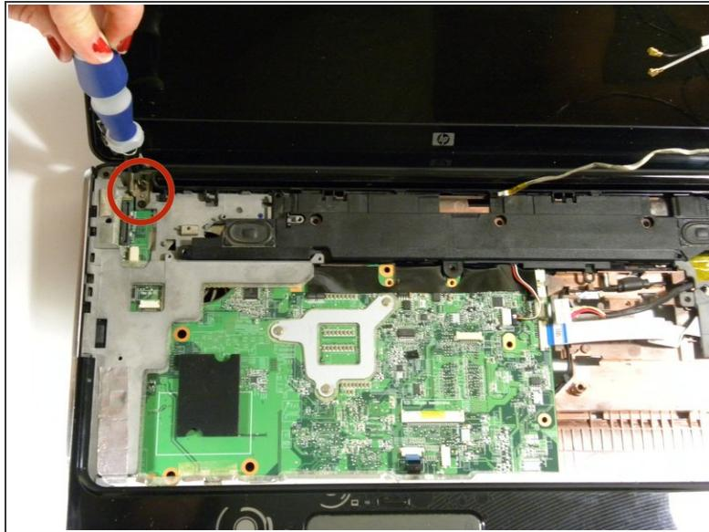
**⚠** Support the display assembly while removing these next screws to avoid damage to the display screen.
